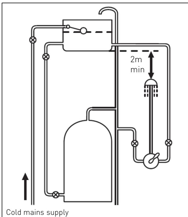
**⚠ Important:** If you install this shower valve with a gravity fed system, there must be a minimum head (vertical distance) from the underside of the cold water storage tank to the showerhead position of at least 2 metres.
