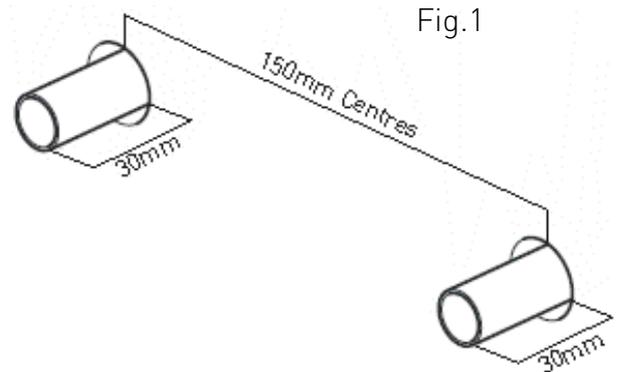
**IMPORTANT:** The water supply pipes to the thermostatic Mixer Valve must be with the Hot on the left and the Cold on the right when viewed from the front.
