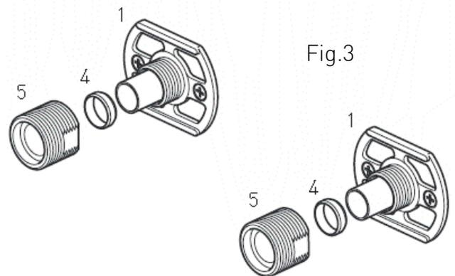
7. Holding the flat edges of the wall plate (1) with a 47mm spanner screw the fixing bridge (5) onto the wall plate (1) using a 22mm spanner. Repeat this step on both sides (See Fig.3).
