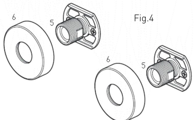
8. Screw the covers (6) over the wall plates / fixing bridges (5), so they are flush against the finished wall surface (See Fig.4).
